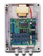
a main supply and power is switched to the relevant outputs as required to control ancillary equipment. An internal transformer reduces the voltage down to 24Vac, 12Vdc and 6Vdc for low voltage equipment such as cameras. The dip switch sets the unique address for each receiver, so that they can be selected from the control keyboard, there is an RS-485 input and output for telemetry connection.
